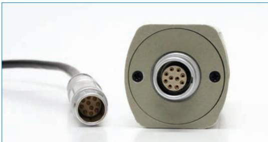
Figure 6. Circular ten-pin connector
