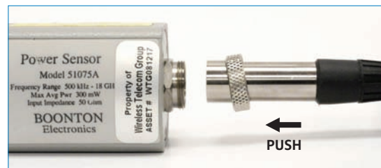
Figure 10. Average sensor connector and sensor cable (open)
