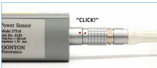
Figure 8. Peak sensor connector and the sensor cable (closed)
