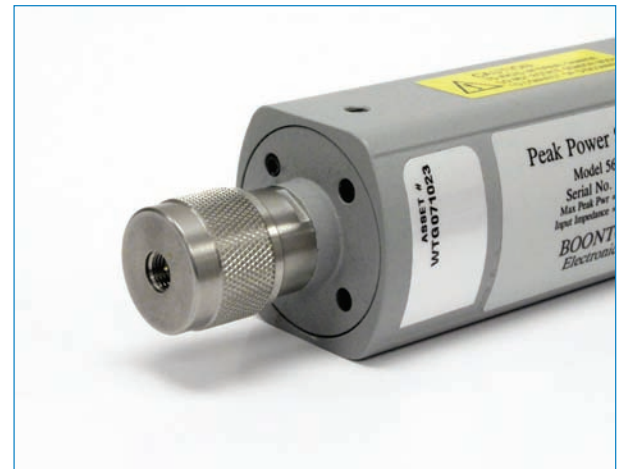
Figure 2. Sensor with K(m) RF connector
